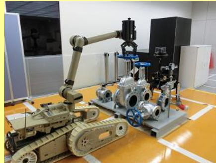
Opening-closing operation of the valve
