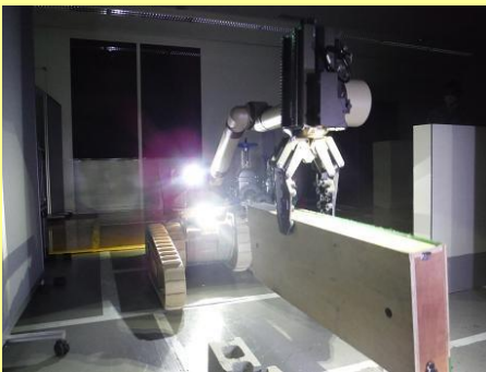
Removing obstacles in the dark
